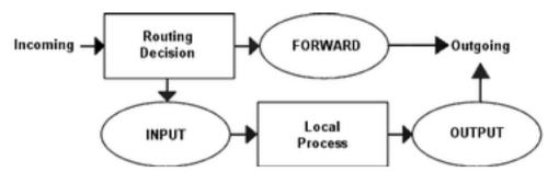
First a routing decision is made, if it's destined for your host, it's sent to INPUT, if it's destined for some box on the localnet it's sent to FORWARD. Then they traverse whichever of those chains. When and if your local box replies to the packets destined for the server, they will traverse the OUTPUT chain.
